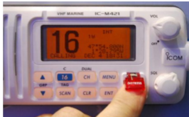
Access to a $1B emergency radio network is as close as the "red button" on your radio.
