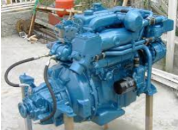
A maritized Perkins 4-236 diesel, which was originally intended to be used in small trucks and tractors. It weighed a svelte 1050 pounds.
