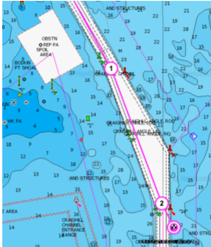
Approximate course of the Ever Forward as she headed south from Baltimore Harbor. At Waypoint 1, a slight course change is required to 161 deg T. At Waypoint 2, a 19 deg course change is required to 180 deg T. The flag shows approximately where she grounded.
